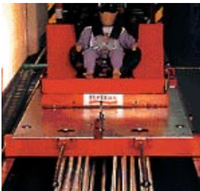
Crash test unit: 22 m/s speed and 784 m/s 2 acceleration, Travel speed
