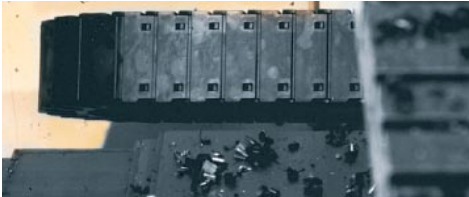
igus® Energy Tubes in the chip area of machine tools
